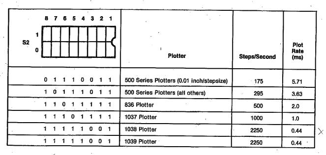
Table 4-2 shows the pulse spacing obtained for each position of switch S2.
