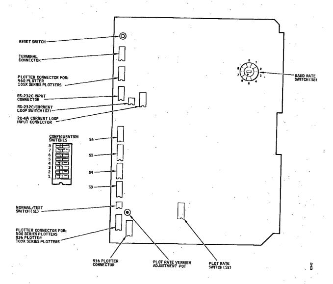
Figure 4-1. CalComp 906 Controller Configuration Switches
